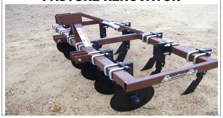
ARMSTRONG AG'S ARMADILLO IS A PASTURE RENOVATOR /AERATOR. The Armadillo uses coulters to slice through the grass mat, followed by shanks to penetrate 4" – 10" into the root zone. This minimizes top ground disturbance leaving a smoother surface.
